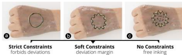
Figure 4: Constraints can be imposed at different levels. In this example, a strict constraint forces the user to closely follow the projected shape primitive (yellow circle, a). A soft constraint allows the user to deviate within a certain margin, for creative adjustments (b). Without constraints imposed, the user can draw freely, while still benefiting from high-level visual guidance (c).
