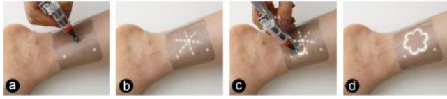
Figure 6: Radial symmetry tool enabling rapid designs of repeating patterns, building on practices from henna art. The user positions the center of the symmetry axes (a), these axes appear as guides (b), the user draws the geometrical pattern in one sector (c), the pattern is replicated in the other sectors (d).
