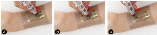
Figure 7: Constraints prevent invalid connections of conductive traces. The user draws a conductive trace to connect two terminals (a). As she is about to connect to another conductive trace and create a short-circuit, the pen retracts to non-inking mode (b). Moving the pen away from the original trace switches the pen back to inking mode (c).
