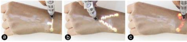
Figure 10: Parametric components. The user places a bend sensor design on the wrist (a) and enhances its visual aesthetic with a curlicue pattern. She drags the center, which modifies the pattern on-the-fly (b). When moving the sensor to a body location the user cannot bend, the body constraint is highlighted in red (c).
