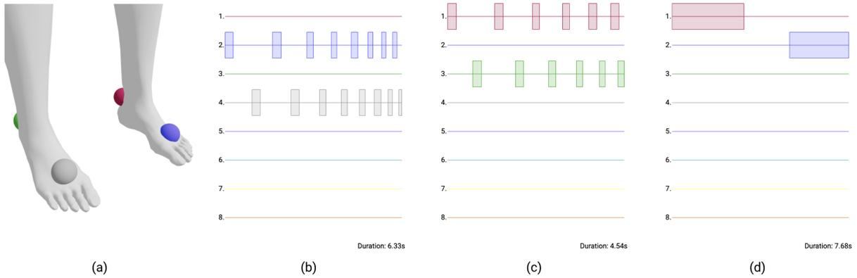
**Tactons in the context of *Bicycling*.** Participants placed the actuators on the feet (a) to provide instructions to the user, e.g. to speed up (b) and (c) or to slow down (d).
