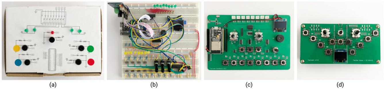
**Figure 2: (a) Initial prototype of *TactJam* used for teaching, (b) breadboarded version of *TactJam* designed for TEI workshop, (c) first PCB version of workshop device and (d) re-designed workshop device with improved ergonomics for bimanual hand-held use.**
